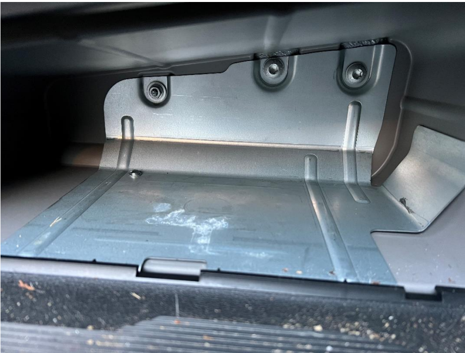
Photo showing the interior of the jack box. The shiny bolt head towards the left is for the clamp seen in the other photo on this page; we located the clamp so that the bolt goes through the metal plate in the jack box (and not just through the plastic, which we worried would not be sturdy).
