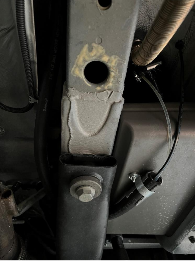
Photo showing rubber heat pipe secured to underside of plastic jack box, then routed forward and then crossing frame piece and turning 180 degrees to head back towards rear.
