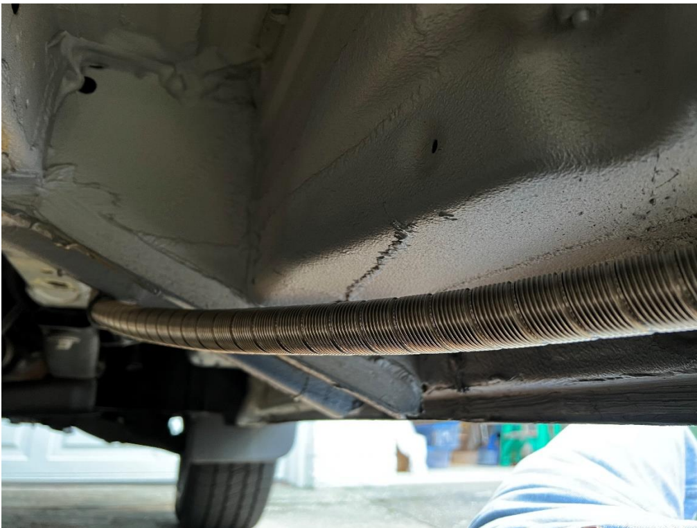
Note the steady downward slope of exhaust line. This shows the section before the muffler.
